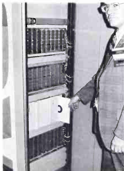
RCA's approach to character generators used computer and floppy disc.
