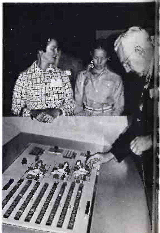
Visual's switcher permitted keyed inserts non-sync remotes while locked to station.
