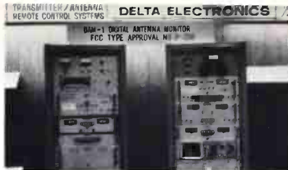
Delta's digital monitor for directional antennas is one of FCC-approved units.
