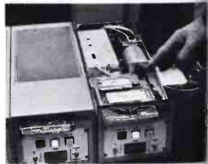
New cart players from Ampro can be installed 3 in a line across rack.
