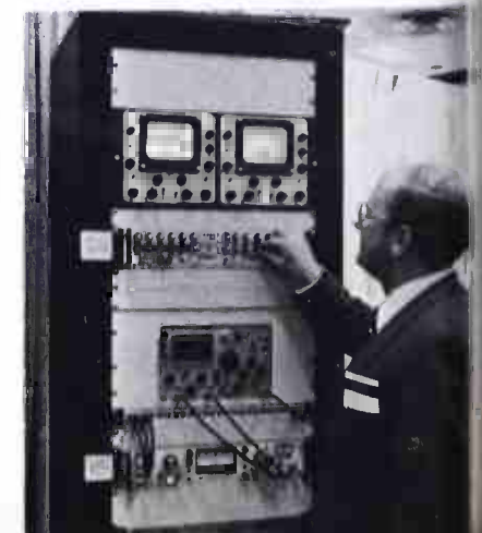
Datatek's phase equalizer, waveform corrector is unit under scopes at top.
